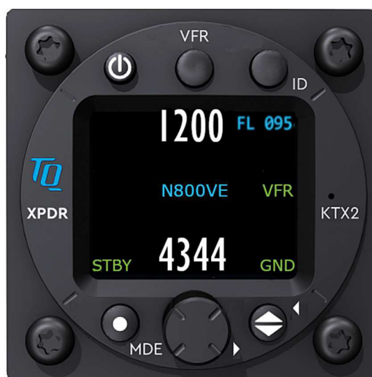
GND-switch installed, on GND
