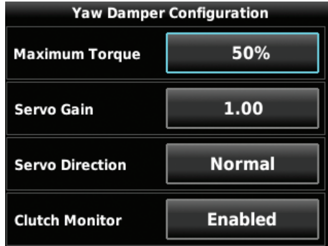
Figure 8-32 Yaw Damper Configuration Page
